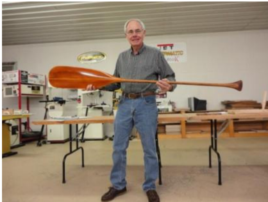
John Freimuth described a paddle he made years ago. The blade is laminated hickory and spruce. The blade is extra big to give a good bite into the water.
