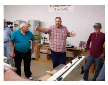
Jason demonstrated a Jet drum sander with an oscillating drum. The oscillation improves finish and sandpaper life. The Jet 22-44 was priced at \$2399.99.
