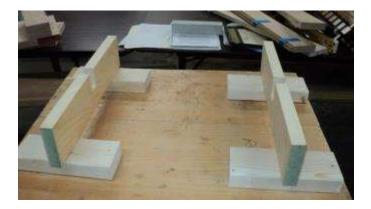
A vertical panel glue up in the fixtures. The technique improves access to both surfaces of the panel to check alignment and to remove/clean up glue squeeze out.
