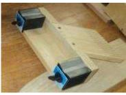
John's second jig makes it easy to accurately replicate ripping out a number of thin strips on a tablesaw/bandsaw. It rides in the miter slot and a moveable indicator locks into position to measure over to the offcut strip or the fence.
