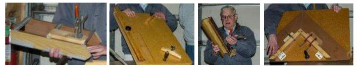
Fixtures left-to-right: Crown molding box for band saw. Table saw cross cut sled for irregular pieces. Crown molding box. Table saw miter sled.
