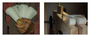
work piece. Applying force with the jaws aligned reduces the potential to damage the work piece and/or the vise. Sure, a "cut off" of the same thickness as the work piece also works but that "rack stop" was neat. Perhaps we'll see a shop built version or two in a future Show & Tell.
